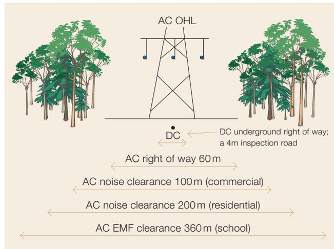
to obtain permits. An underground DC cable naturally has no audible noise emission.
